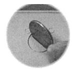
Before attempting to transport your scanner, it is important that you lock the optical assembly in place to avoid any possible damage to the scanner's optical components. To lock the optical assembly, insert a coin and turn it until it points to the lock mark.
